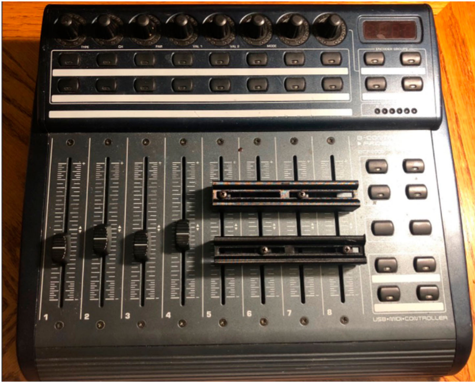
Figure 6. Picture of 3D-printed dual fader caps used on the Behringer BCF2000.
